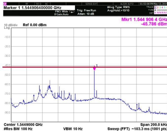
Figure 5.3: Glonass-K SAR Repeater L-Band Downlink Wide Band Signal Spectrum
