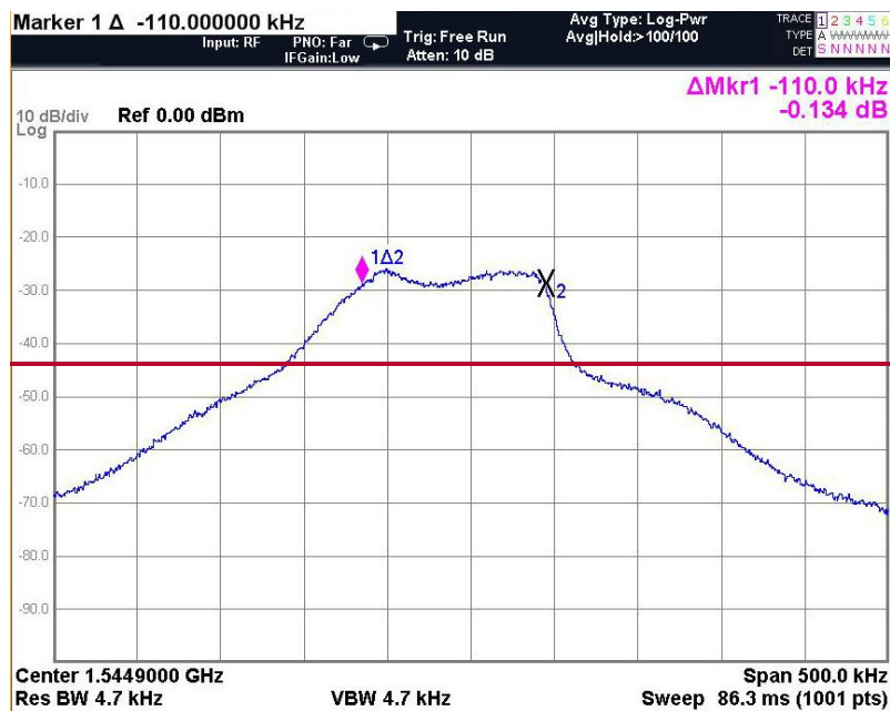
Figure 5.6: Glonass SAR Repeater Normal Bandpass Filtering Performance
