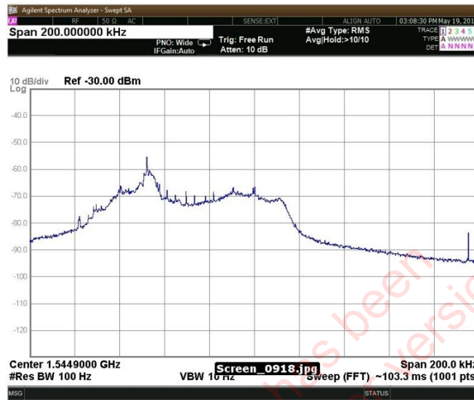
Figure 5.2: Glonass-K SAR Repeater L-Band Downlink Narrow Band Signal Spectrum
