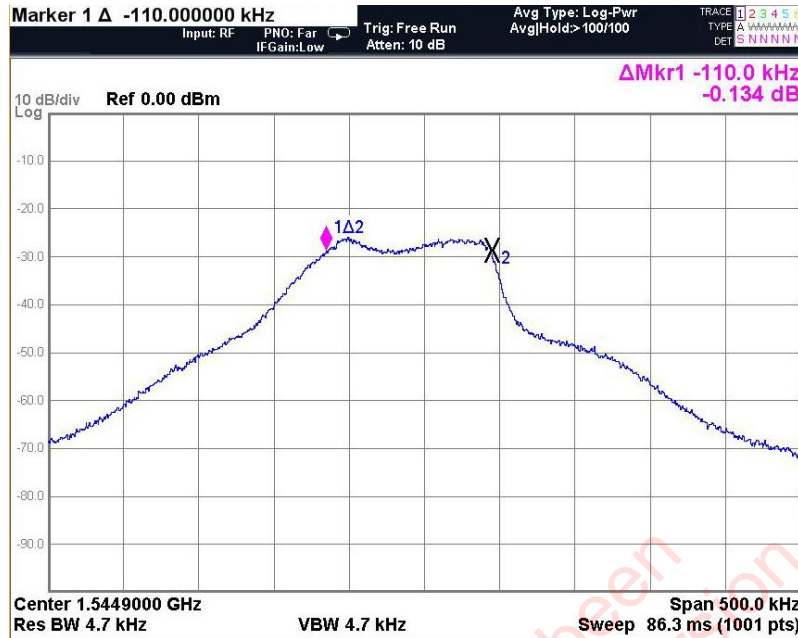
Figure 5.6: Glonass SAR Repeater Normal Bandpass Filtering Performance
