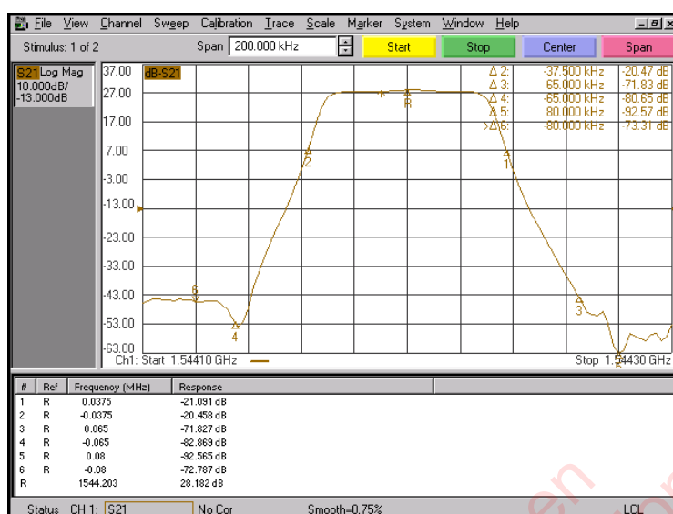
Figure 6.3: BDS MEOSARR Narrow Band Spectrum Characteristics
