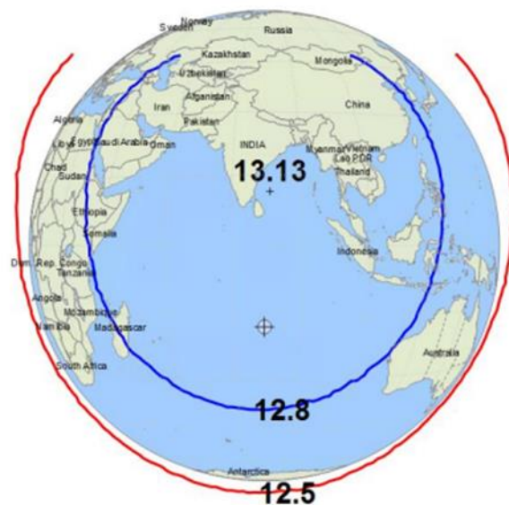
Figure 4-11: INSAT-3DS SASR 406.05 MHz Receive Antenna Contour Pattern
