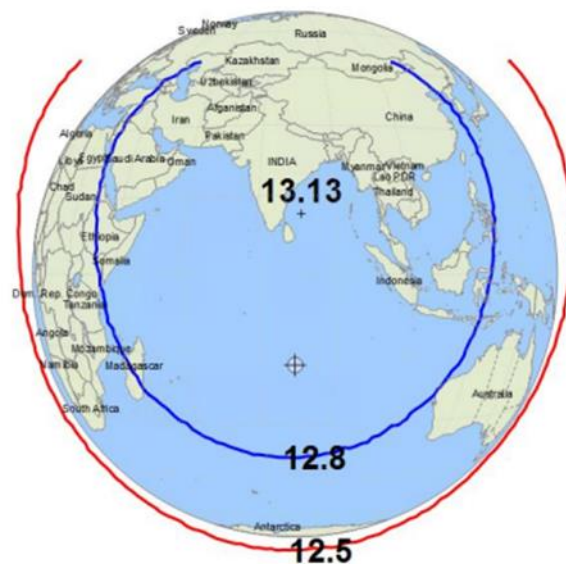
Figure 4-11: INSAT-3DS SASR 406.05 MHz Receive Antenna Contour Pattern
