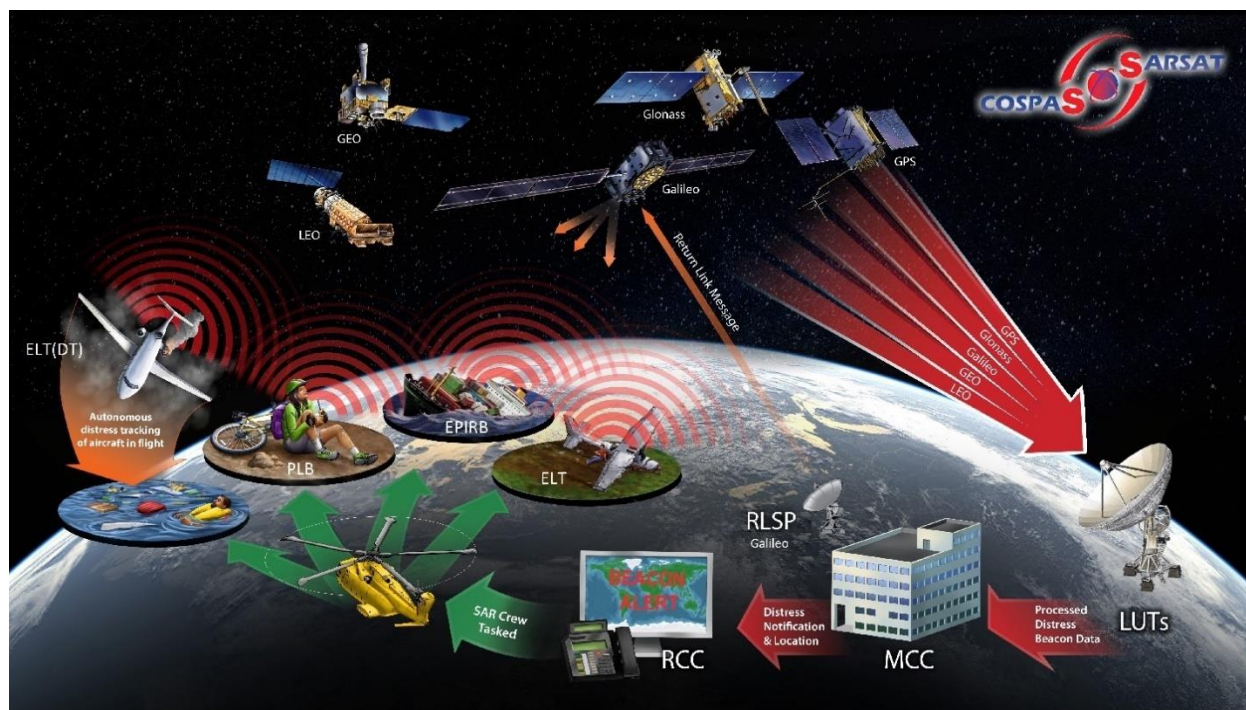
Figure 8: Cospas-Sarsat System Overview
