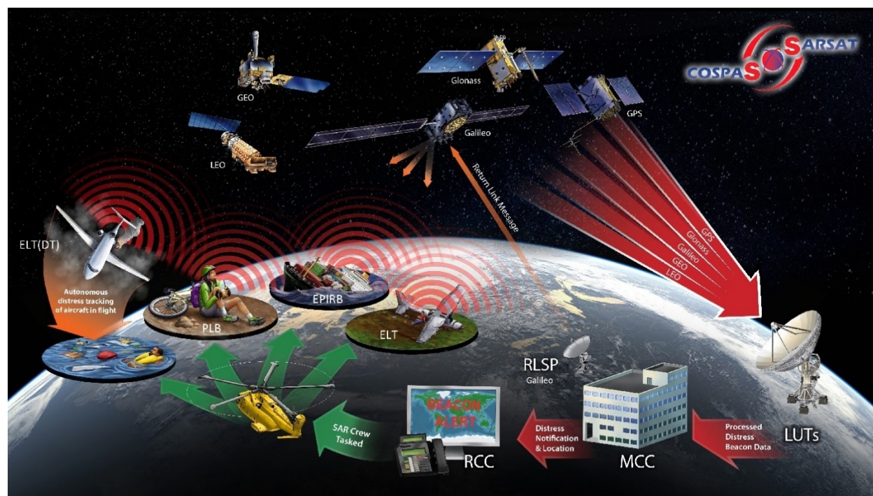
Figure 8: Cospas-Sarsat System Overview
