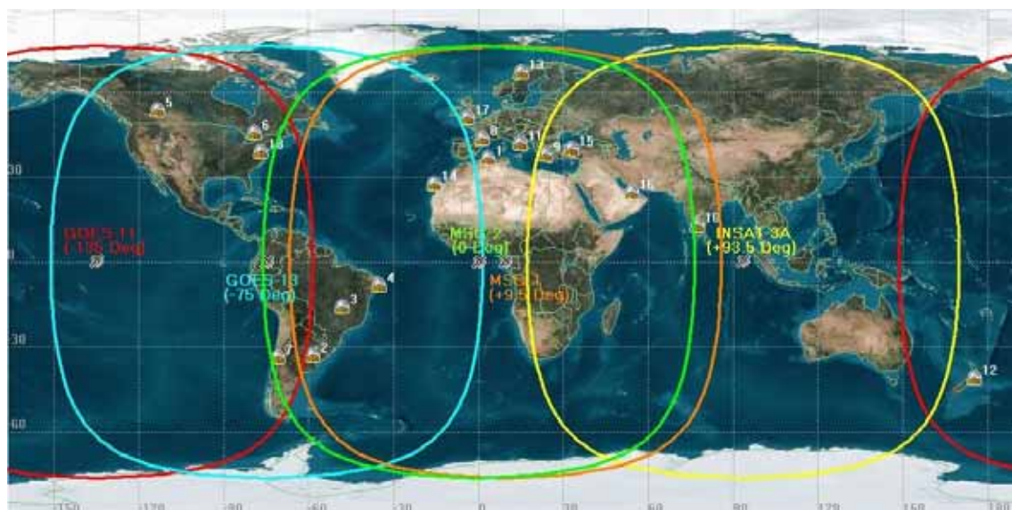
Figure 6: GEOSAR Satellite Coverage and GEOLUTs (December 2010)
