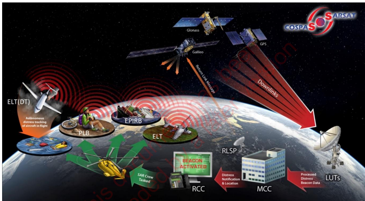
Figure 3.3: An Overview of the MEOSAR System
