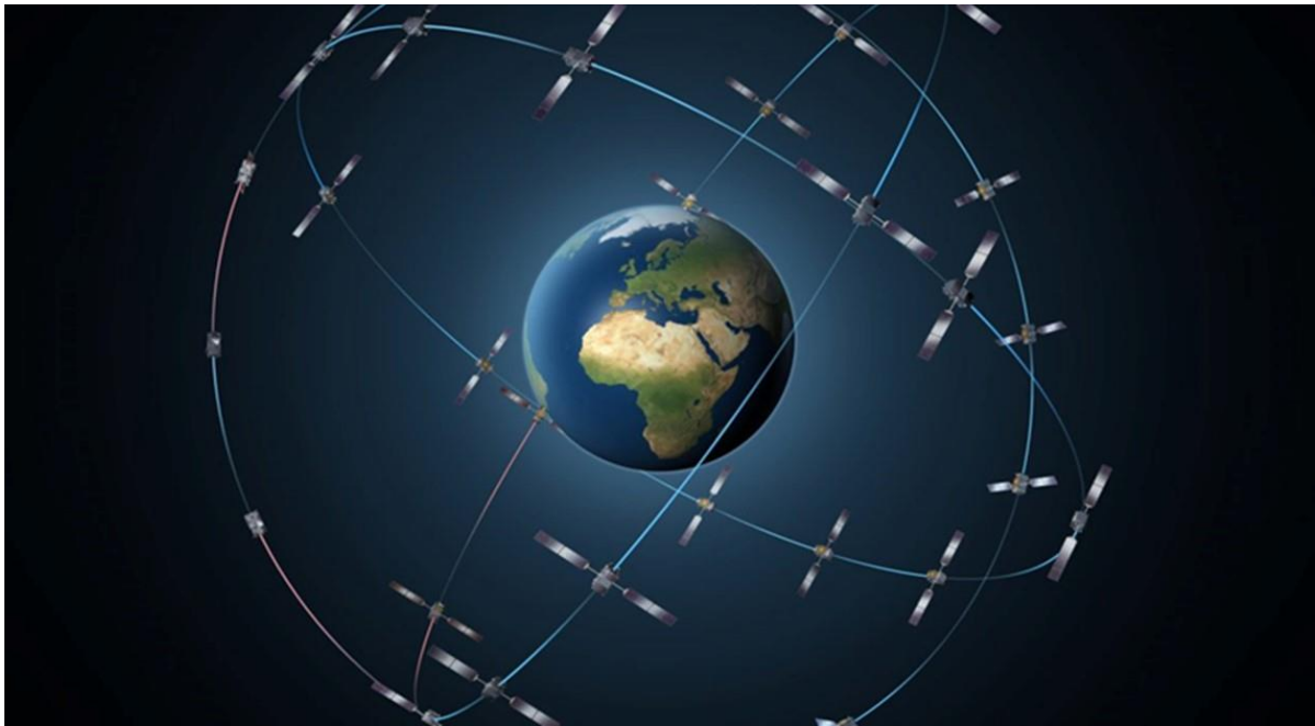
Figure 3.1: A Schematic View of the Galileo Constellation (which is one of the constellations of the MEOSAR System)
