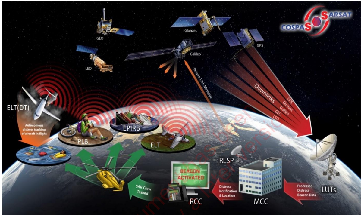
Figure 1.1: An Overview of the Cospas-Sarsat Beacon Detection System
