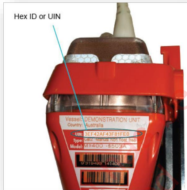
Figure 2.3: Beacon with Hex ID 3EF42AF43F81FE0
