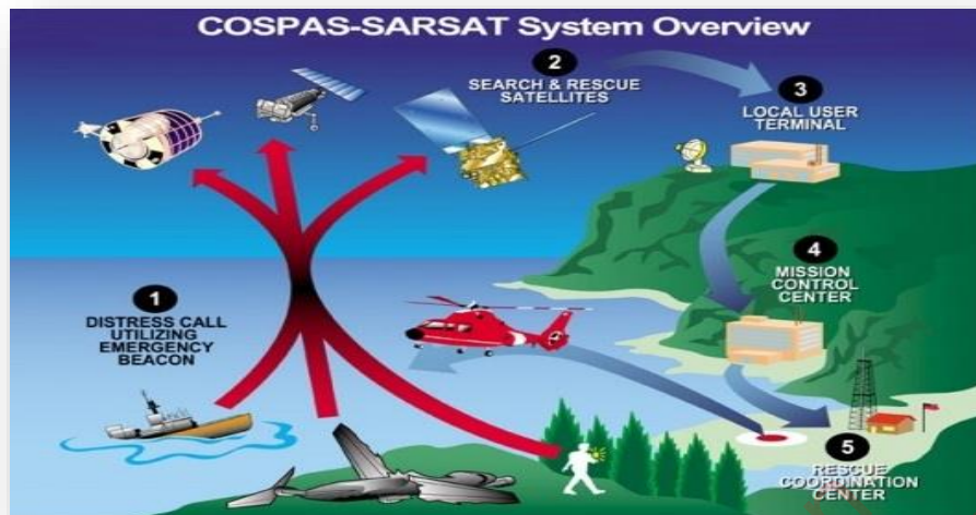
Figure 1.1: An Overview of the Cospas-Sarsat Beacon Detection System
