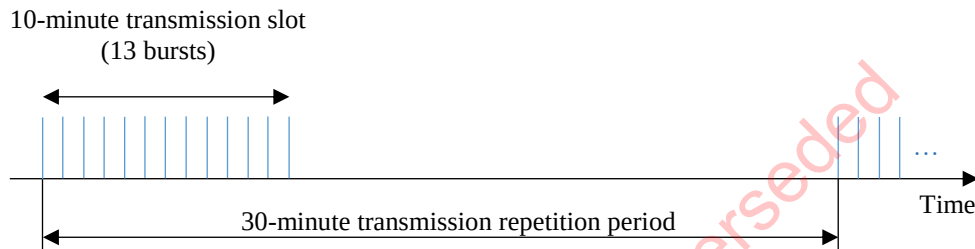
Figure 2.1: Definition of the Transmission Repetition Periods
