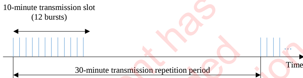
Figure 2.1: Definition of the Transmission Repetition Periods
